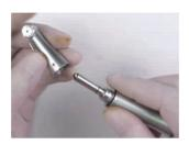
6. Twist the screw with 2# tooling.
