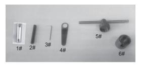
2. Fix the head with the small side of the opening slot of 4# fixture, align the slot of the handle with 3# fixture and unscrew the handle.
