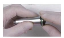
4. Install the gasket on the movement (note: the front and back of the gasket, with the bump pointing outwards), then assemble the movement into the head, and twist the rear cover of the movement with # 2 tooling.
